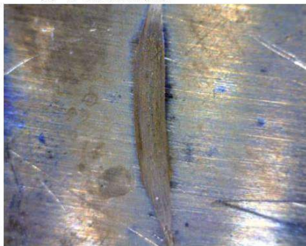
(a) Wear track (RT):
